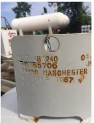
If you have a DOT propane tank, it must be re-qualified after 12 years of manufacture date. Smaller portable propane tanks from 5 lbs to 420 lbs or 1 gallon to 120-gallon tank can be transported over the highways and roads are regulated by The Department of Transportation. If it is a DOT tank, it will be stamped on the outside collar of the tank. It will say "DOT-"
